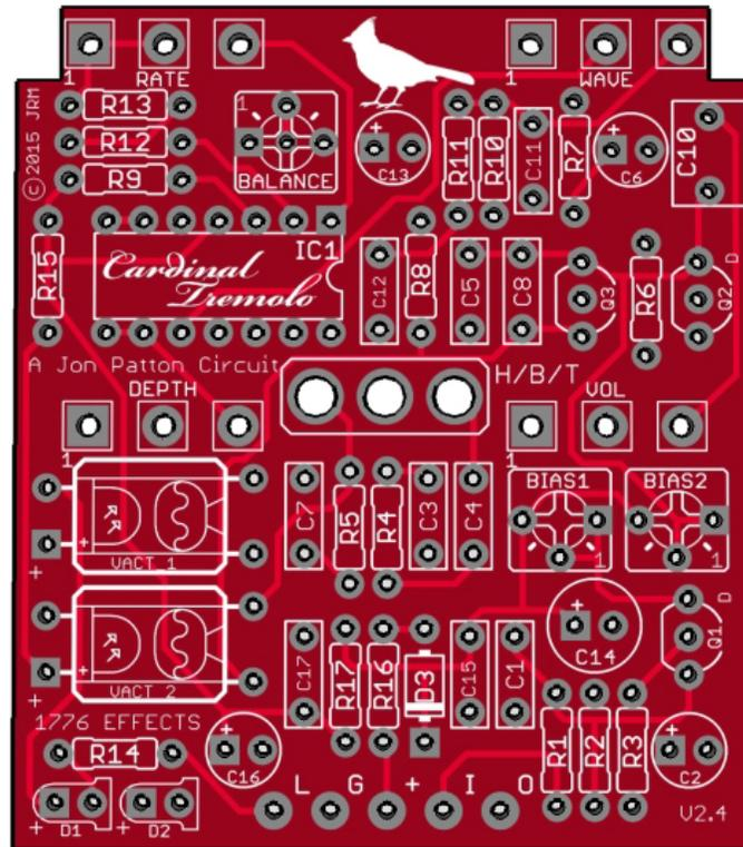
The Cardinal Tremolo is a transistor and vactrol implementation of the Harmonic Tremolo. It resembles the harmonic tremolo from Fender's 1960-1963 amps; the Super, Pro, Twin, Showman, and Concert models.
